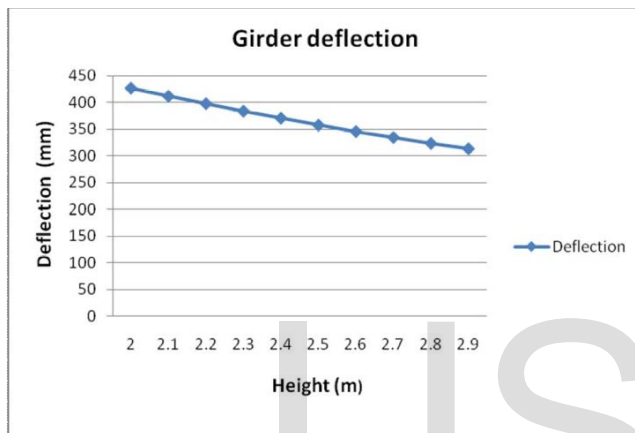
Fig 5: comparison of girder deflection and height of girder.
