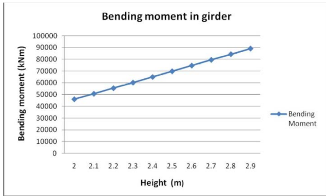
Fig 4: comparison of bending moment and height of girder.
